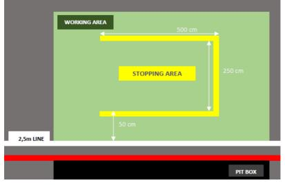
When the car is stopped, in its dedicated stopping area, no part of the car must cover the longitudinal lateral tape defining the area in top view.
