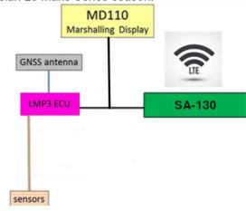
This mandatory use results in the addition of the following elements in the articles below of the 2025 LMP3 technical regulation:
